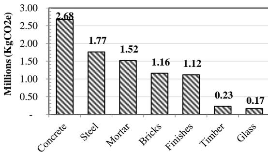
**Fig (2) CO<sub>2</sub>-equivalent emission from building components**
