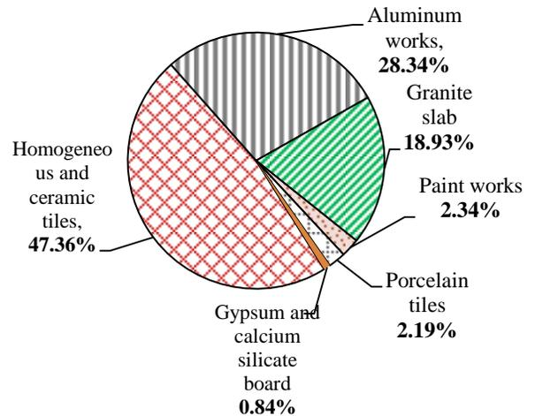
**Fig (5) Major embodied carbon emission of finishes components**
