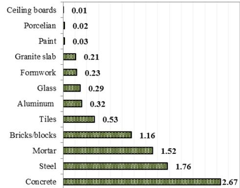
**Fig (4) Total carbon emission form building components**
