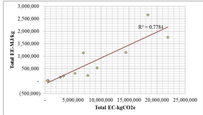
Fig (9) Correlation co-efficient between embodied carbon and embodied Energy
