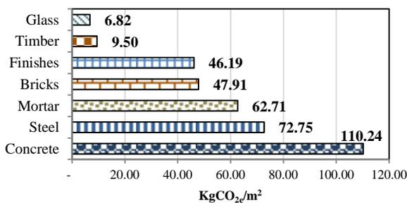
Fig (8) Contribution of carbon emission per (GFA) m<sup>2</sup>
