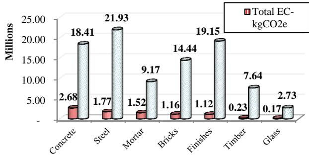
Fig (6) Comparison of embodied energy and embodied carbon
