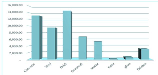
Fig (7) Carbon emission from materials transportation
