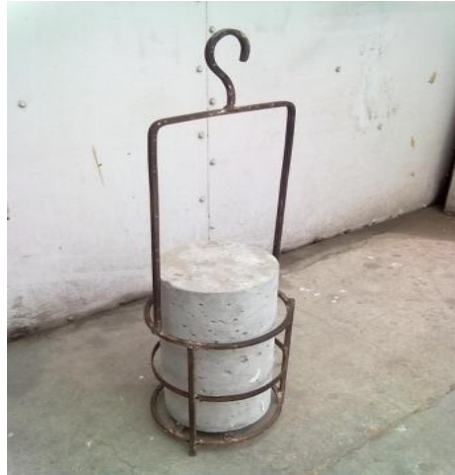
Figure-3 Cage used to dip concrete cylinders in boiling water Table 4: Description of the concrete mixes
