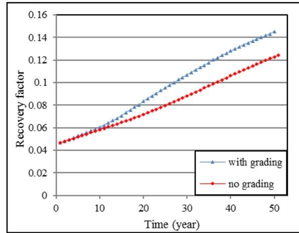
Fig 7. Recovery factor for N<sub>2</sub> injection
