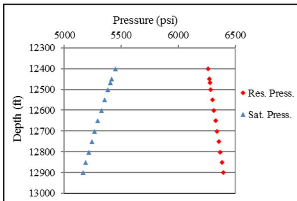
Fig 4. Effect of compositional grading on saturation pressure
