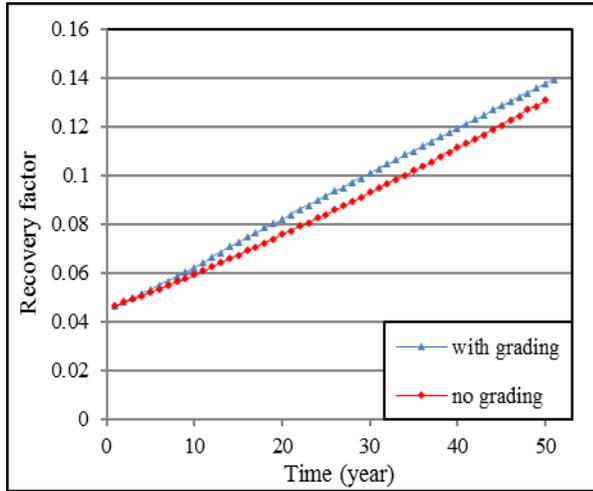
Fig 10. Recovery factor for CO<sub>2</sub> injection, injection rate = 10 MMSCFD, production rate = 1500 STBD
