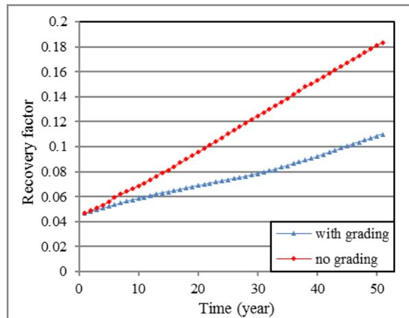
Fig 9. Recovery factor for separator gas reinjection
