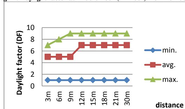
Fig.12: Daylight factor at upper floor for 18 storey.
