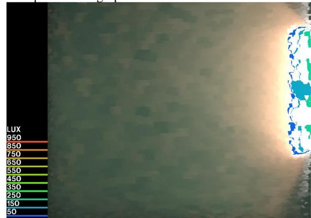
Fig.7: Illuminance reading from window distance at lower unit with 3m building separation.
