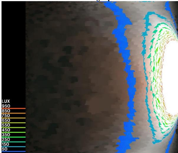
Fig.9: Illuminance reading from window distance at lower unit with 30m building separation.
