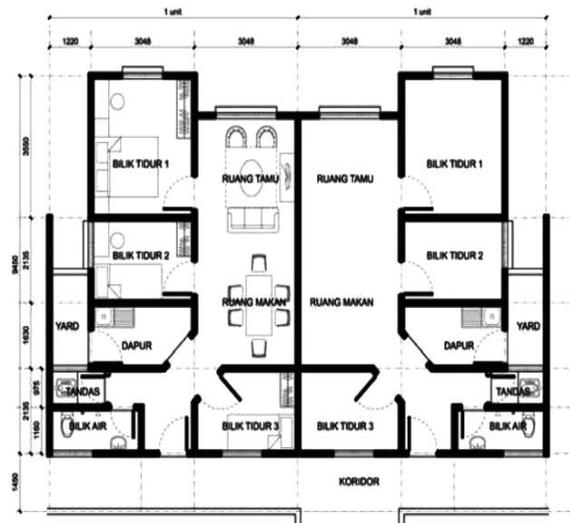
**Fig. 2: Standard unit layout plan (typical domestic unit) for 18-storey low cost flats.**
