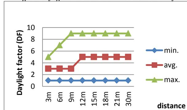
Fig.11: Daylight factor at middle floor (9th floor) from 18 floors.
