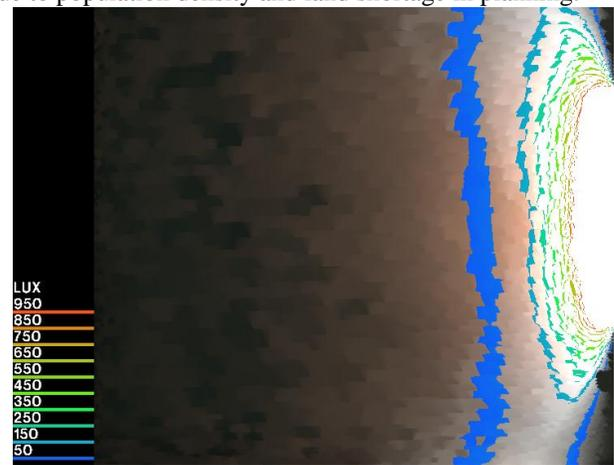
Fig.6: Illuminance reading from window distance at lower unit with 24.4m building separation referring to planning guideline.
