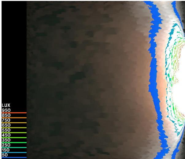
Fig.8: Illuminance reading from window distance at lower unit with 15m building separation.
