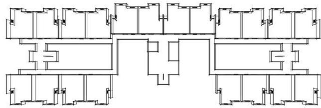
**Fig.1: Standard typical storey plan for 18-storey low cost flat.**
