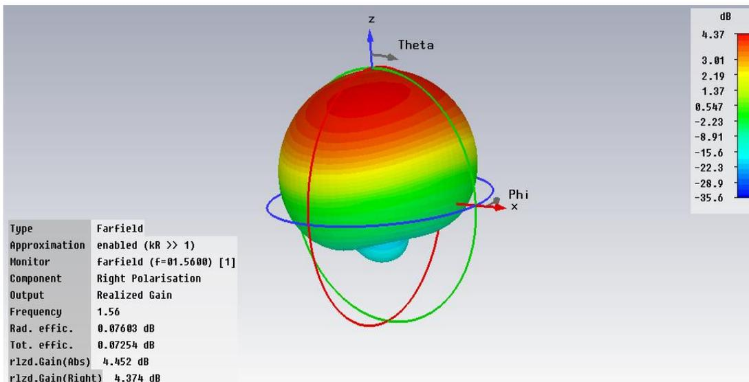
Figure 7. Right-hand polarized antenna pattern
