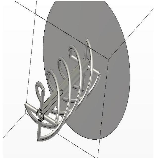
Figure 2. 3D of the final antenna model
