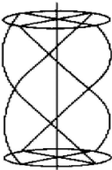
Figure 1. Resonant four-arm spiral antenna
