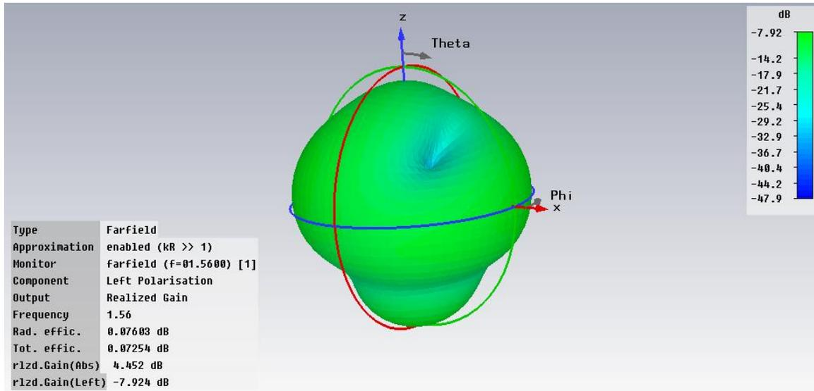
Figure 8. L-polarized antenna pattern
