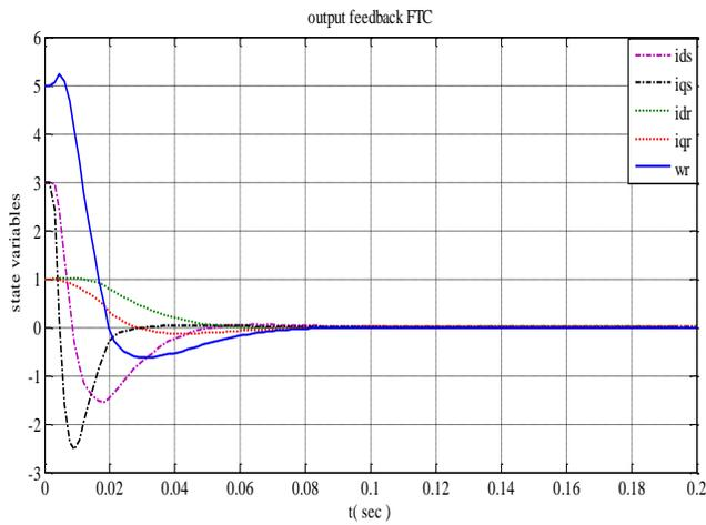
Figure 3. Responses of TPIM under the fixed output feedback FTC for normal mode.
