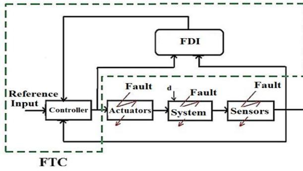
Figure 1. The closed-loop system with FTC and FDI
