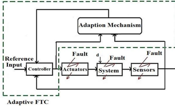
Figure 2. The closed-loop system with adaptive FTC
