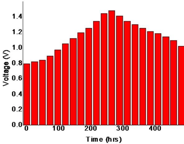
Fig.2: Generation of voltage from Sewage wastewater with Potassium permanganate and Carbon rod
