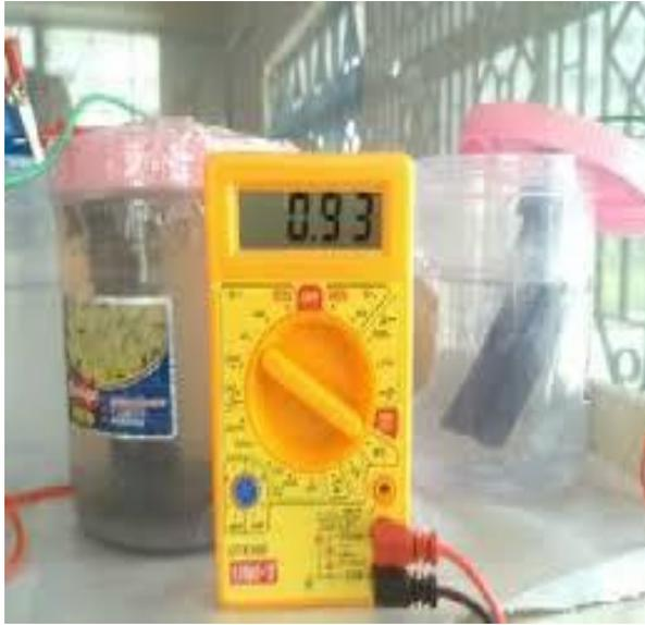
**Fig. 1: Microbial Fuel Cell set-up using Salt-bridge**
