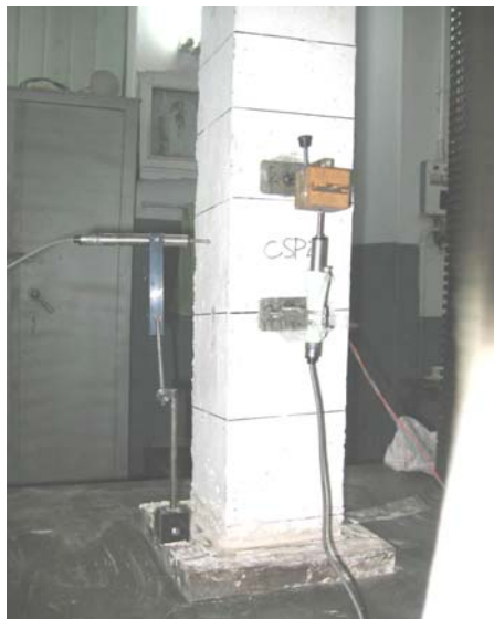
Fig 11: LVDTs Installed for Measurements of Horizontal and Vertical Deformations
