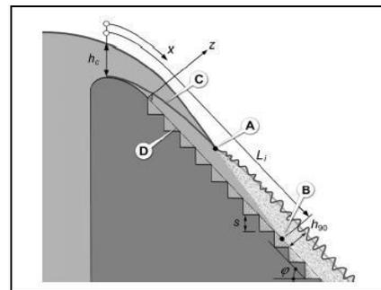
Fig (2) Stepped Spillway [2]
