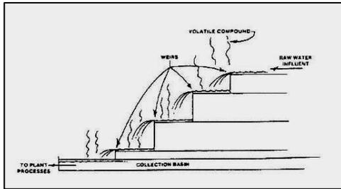
**Fig (4) Process of stepped spillway/cascade aerator [4]**
