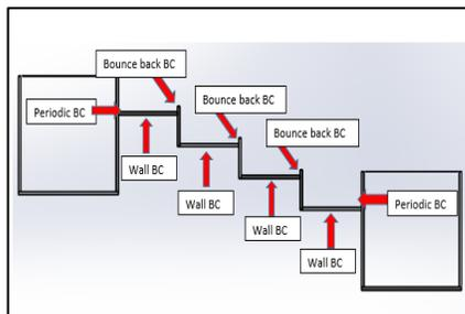
**Fig (8) Periodic Boundary Condition Diagram**
