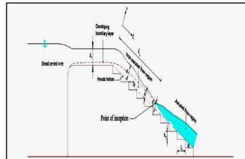
Fig (3) Non-aerated and aerated flow region in skimming flow. [3]
