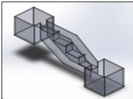
**Fig (5) Schematic diagram of stepped spillway**
