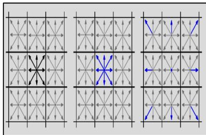
**Fig (7) Collision-Propagate scheme for the D2Q9 model. [8]**
