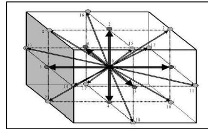
**Fig (6) Lattice arrangement for D3Q19. [7]**
