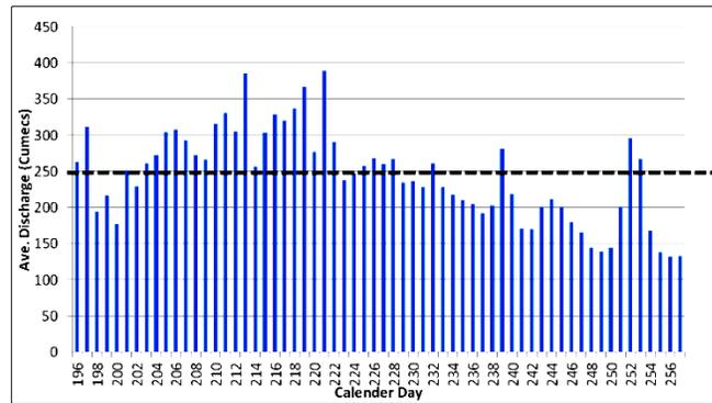
Fig 18. Average Discharges During Second Flood Period between 15th of July (196) and 15th of September (257)
