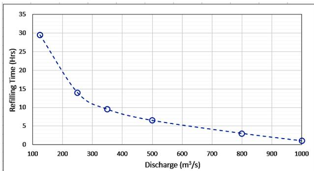
**Fig. 20: Time required refilling the reservoir with different discharges**
