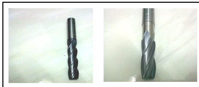
Figure 2: The physical comparison of the long series/full flute and ground shank end mill
