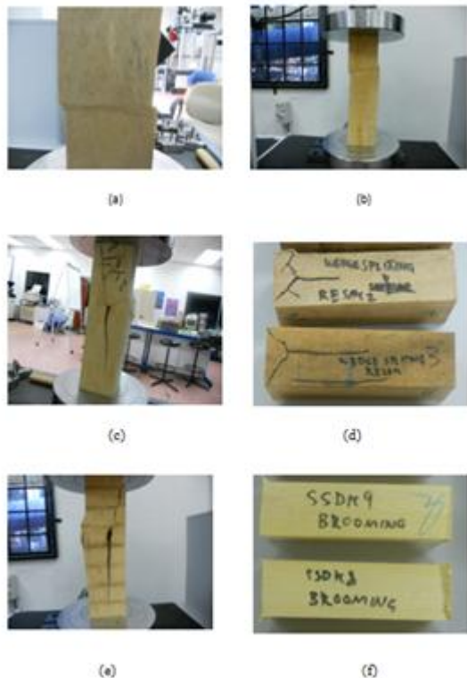
Fig(4) Characteristic of Compression Failure: (a) crushing (b) shearing (c) crushing and splitting (d) wedge splitting (e) splitting (f) brooming
