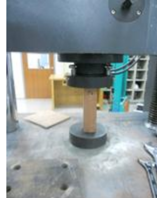
Fig (3) Compression Test Set-up for Small Clear Specimen
