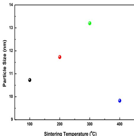
Figure 2. XRD particle size as a function of sintering temperature.
