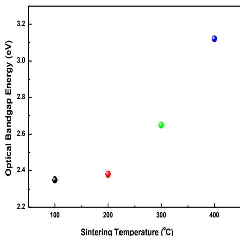
Figure 5. Optical direct bandgap energy as a function of sintering temperature.
