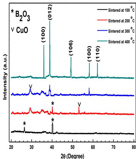
Figure 1. The XRD patterns of the all samples sintered at different temperatures.
