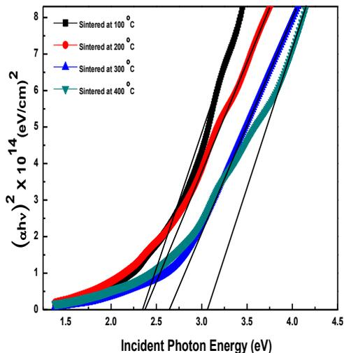
Figure 4. The optical direct bandgap energy of all prepared samples.
