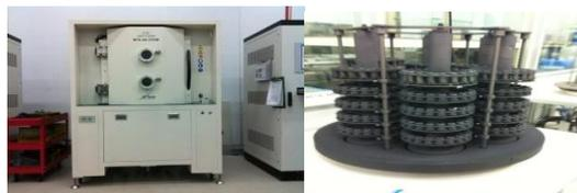
**Figure 1:** (a) PVD Arc system technology constructed by J&L technology Korea, Model Legend H.I.P. III. (b) Substrate holder outside the coating chamber
