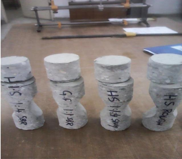
Figure 2 Failure of the cores in tensile test
