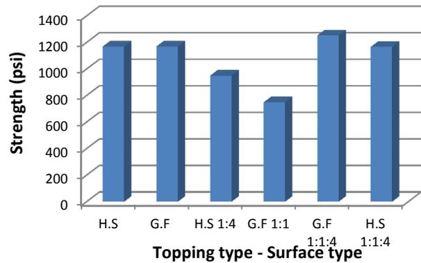
Figure 4 Compressive strength of cores
