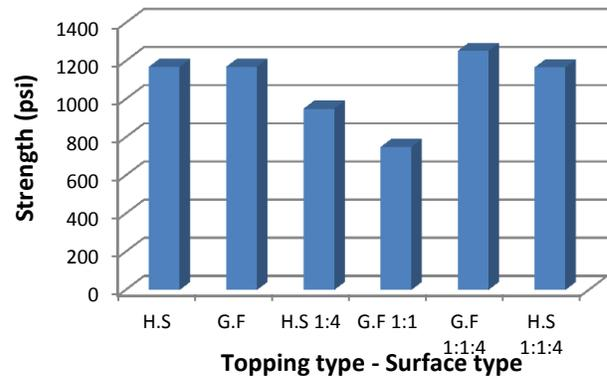
Figure 4 Compressive strength of cores
